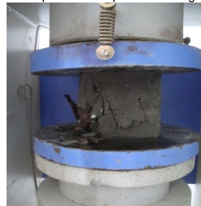
Fig. 1. Set-up for the compressive strength test.
